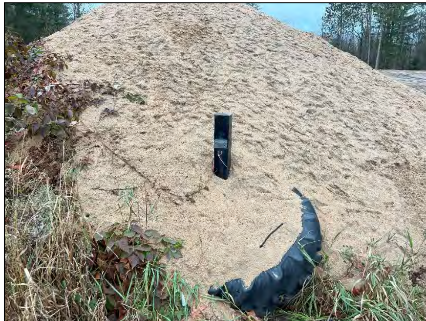
PHOTO 6 – MW4 Covered in Sand since Spring 2023 – (Fall 2023, Facing East)
